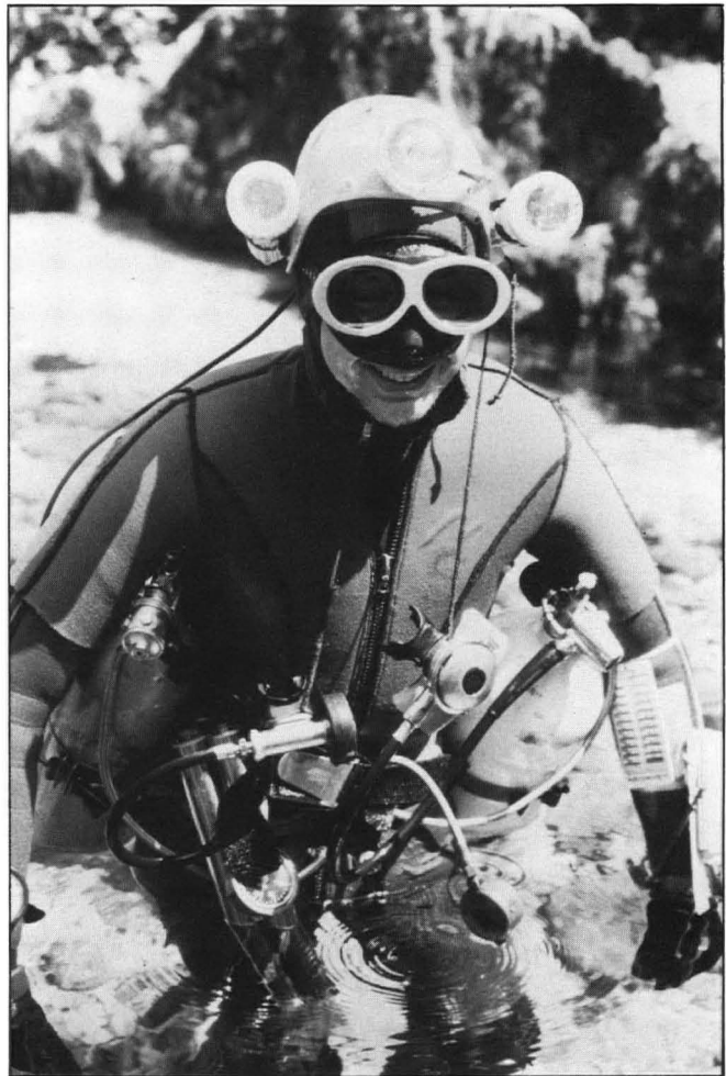
A well equipped cave diver with two independent breathing supplies, three lights, navigation equipment and two decompression slates (Photo: J Cordingley).
